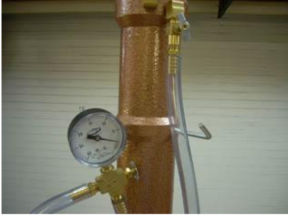
5. Attach vacuum gage to tower vacuum supply using vinyl hose.
