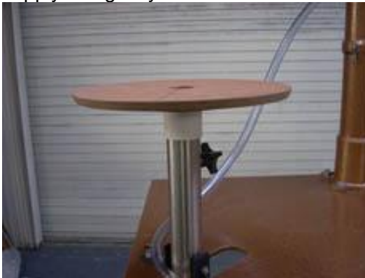
5. Attach vacuum gage to tower vacuum supply using vinyl hose.
