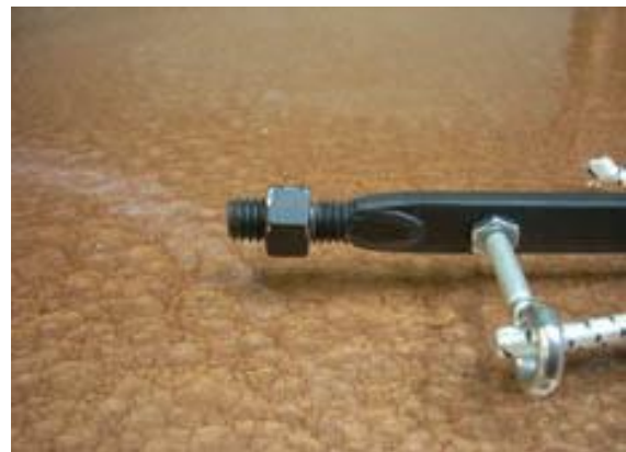
2. Adjust locking nut on outrigger attachment threads.
